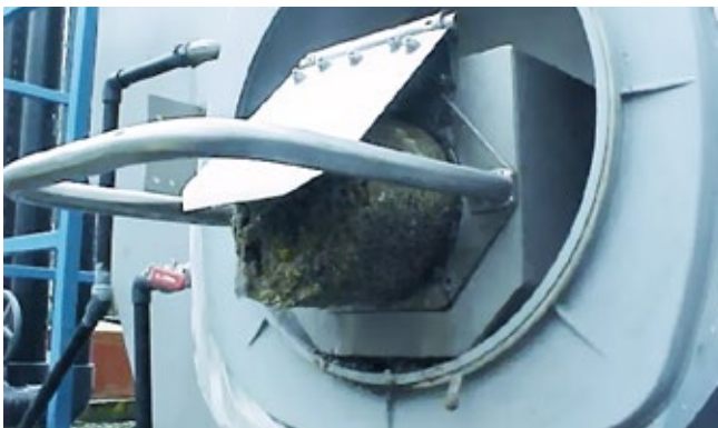
An efficient screw compactor for easy transport of waste
