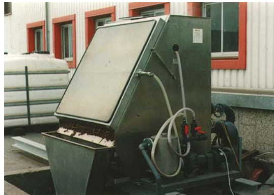
Slaughterhouse raw sewage - Stainless 554 - 48" frame. Rotating front and rear spray system with cover.
