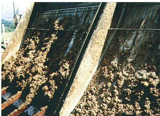
Thickening of paper millstock. 2 x 48" stainless 554 frame.
